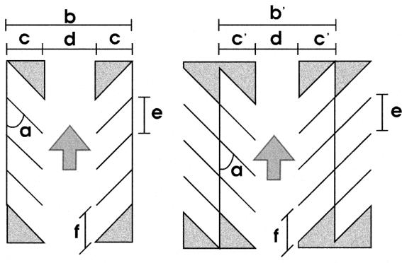
a Parking Angle b/b' Parking Section Width c/c' Parking Bank Width d Aisle Width e Curb Length Per Car f Car Stall Width
