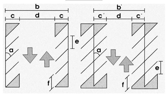
a Parking Angle b/b' Parking Section Width c/c' Parking Bank Width d Aisle Width
